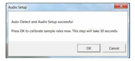
3.2.8 Press **"OK"** to calibrate the Audio device sampling rate. Calibration of Sample rate takes approx 30 seconds.
