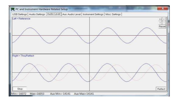
3.2.10 Next connect the TX port to the RX Port with a short Coax cable. The sine-wave on the Right = Tru/Reflect should now disappear (because the TX port is now terminated with a 50 Ohm load from the RX port).
