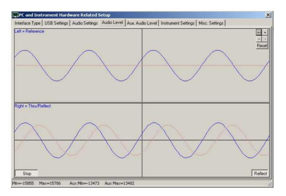
3.4.12 Next connect the TX port to the RX Port with a short Coax cable. The sine-wave on the Right = Tru/Reflect should now disappear (because the TX port is now terminated with a 50 Ohm load from the RX port).
