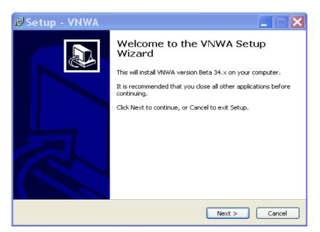
3.3.3 Press "Next >" – The default location where VNWA will be installed will be shown: Note: Select a different Destination Location (ie C:\VNWA 2) if you want to install a second VNWA application on the same PC. This prevents overwriting the set-up files of your first VNWA application.
