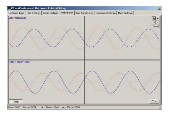
3.4.14 This step is **only for VNWA 3E** with fitted expansion board: Select Tab **"Aux Audio Level"** and screen below should be displayed. (RX port is receiving TX output via Thru coax cable).
